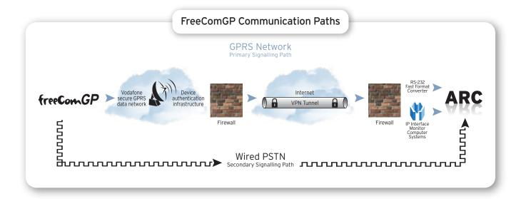
FreeComGP is the perfect replacement for standard intruder digital communicators, as well as ideal for new installations. It uses Vodafone UK's secure GPRS network as its primary signalling path to send alarm signals as packet data. A standard PSTN telephone line is used for backup in case the mobile data network is unavailable.
